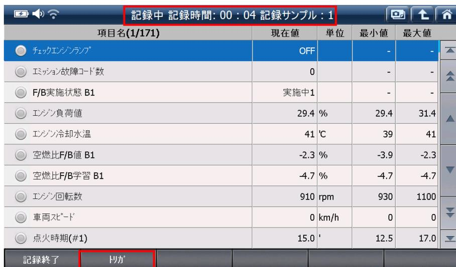
The screenshot shows the '記録中' (Recording) screen. The status bar at the top indicates '記録中 記録時間: 00 : 04 記録サンプル : 1'. The background table shows the current values for the same engine parameters as in the previous screenshot. A 'トリガ' (Trigger) button is highlighted in red at the bottom.
