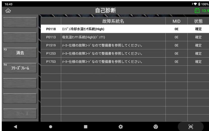
The screenshot shows a mobile application interface for OBD-II diagnostics. The title is "自己診断" (Self-Diagnosis). The time is 16:43 and battery is at 100%. A table lists the following fault codes:
